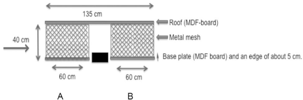
**Figure 3.** Set-up design of influenza virus (H3N2, Pan/99) aerosol-transmission experiments between guinea pigs. Guinea pigs ( $n = 4$ ) were intranasally infected with  $5 \times 10^3$  pfu of Pan/99 virus in 100  $\mu$ L (50  $\mu$ L in each nostril). All four infected animals were placed into an experimental cage “A”. At 30 h p.i. four naïve uninfected guinea pigs were placed in cage “B”. Air-flow from left to right. Air exchanged 17x/day. Filled rectangle = ionizer.
